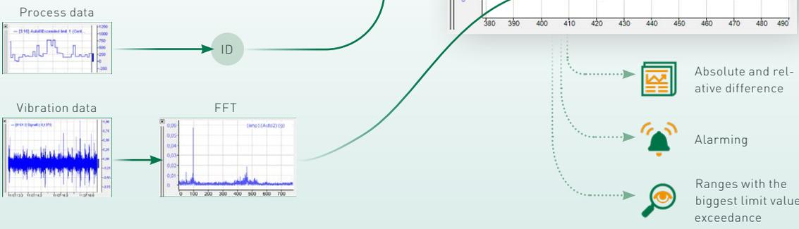
Example of monitoring with the ibaInSpectra Auto-Adapting module
